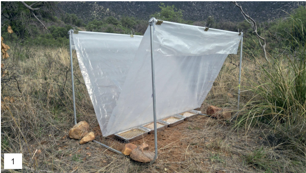
Figs. 1-2. Photos of V-FIT traps (both taken from Löbl et al. 2021): 1- V-flight intercept trap, with metal frame; 2- travel version of V-flight intercept trap.
